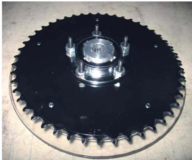
9. Then slide the smaller sprocket onto the bolts with the bevel side of the teeth facing the other chainring. The goal here is to separate the chains as much as possible.
