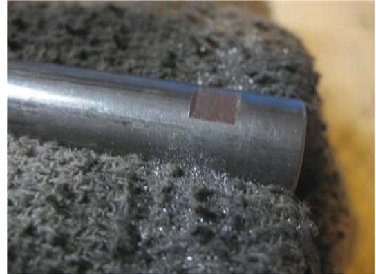
The flats do not have to be large but should be wide enough to allow lateral adjustment. Once this step has been completed reassemble the jackshaft like before.
