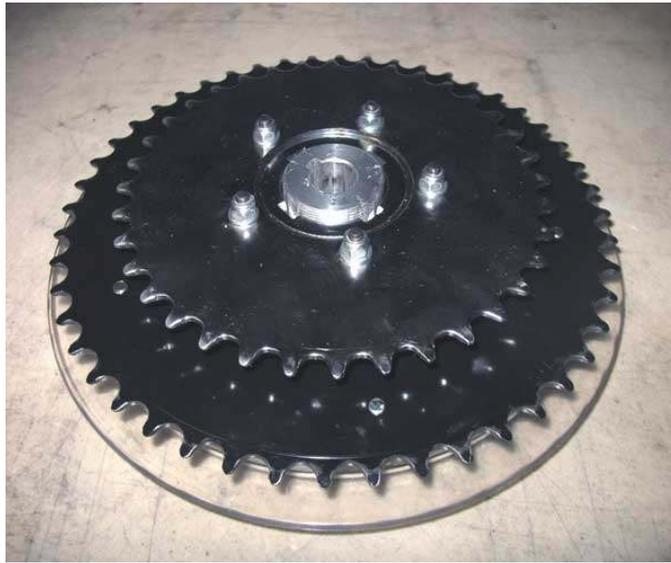
10. Tighten the chainring assembly with the 5 locknuts and washers. Be sure that the bolts are tight against the outer chainring before installing the locknuts.
