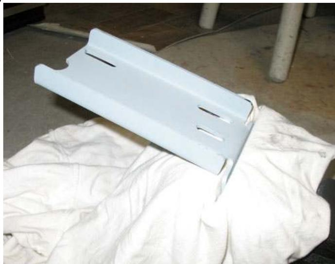
2. Assemble the front mount plate to the motor mount using one of the 6 mm cap screws, flat washer and lock washer. Do not fully tighten this bolt. The two plates should be able to slide on the adjuster slot.
