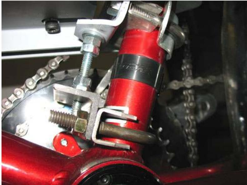
3. Add 1.5 inches to your measurement and cut the adjuster rod to that length.
