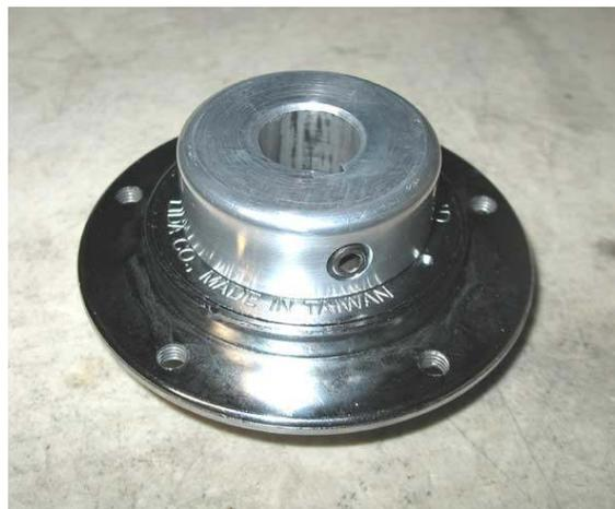
4. Test fit the freewheel hub and freewheel to the crank spindle with the supplied key. Make sure that they fit and can be slid along the shaft to allow for adjustment later.
