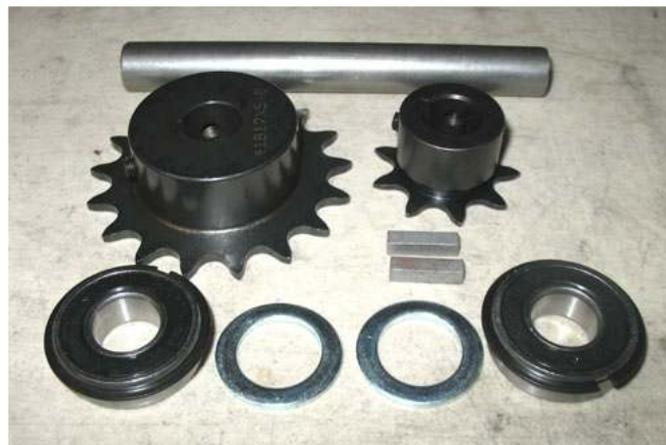
Sand and file the shaft, sprockets and keys as necessary so that they can easily be assembled and disassembled by hand. As we fit these pieces together they will need to be easily slid along the shaft for adjustment and disassembly.
