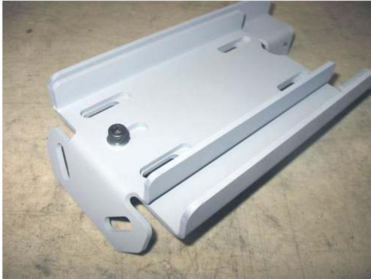
3. Assemble the rear mount to the motor mount using the 6 mm hex head bolts, washer and lock nuts. Insert the bolt from in between the rear mount and install the washer lock nut to the outside. Repeat on the other side. The chain adjuster tab should be below the mount. Do not fully tighten these yet. The rear mount should be able to rotate on the bolts. Note the 2 cap screws are put in the rear slots just to keep things aligned as we continue assembly.
