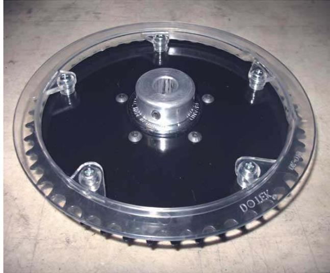
8. Next place the 5 spacers (6mm nuts) over the bolts up to the freewheel.
