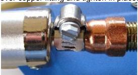
Optional method: Install muffler per step one, drill a small hole (~ 3/32") through copper fitting and insert cotter pin:
