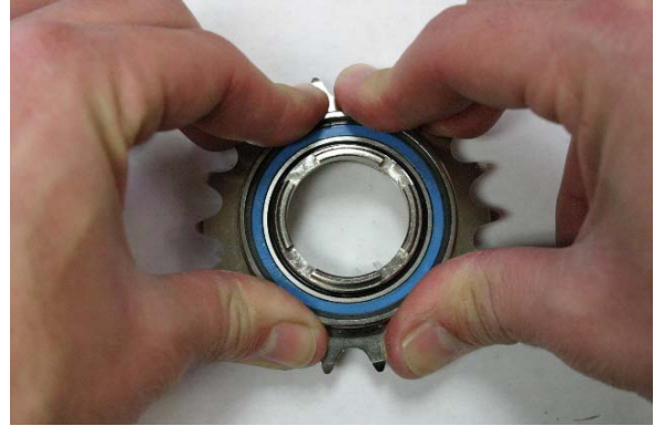
Fig. 19 Press down to seat inner driver.
