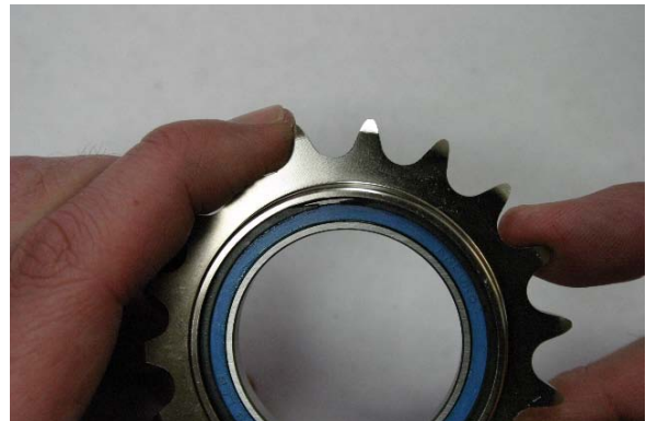
Fig. 17 Snap ring seated properly.
