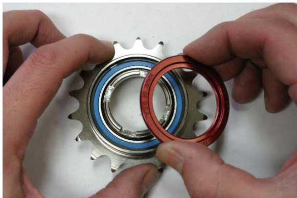
Fig. 20 Install lock ring.
