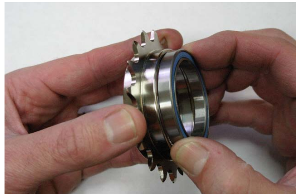
Fig. 11 Start bearing into bore.
