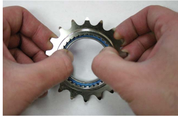
Fig. 9 Pressing out bearing.
