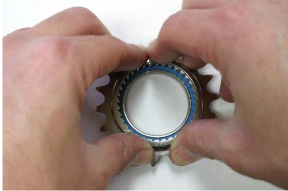
Fig. 12 Pressing bearing into bore.
