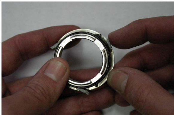
Fig. 7 Checking pawls of inner driver
