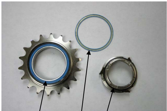
Fig. 6 Bearing, rear seal, inner driver
