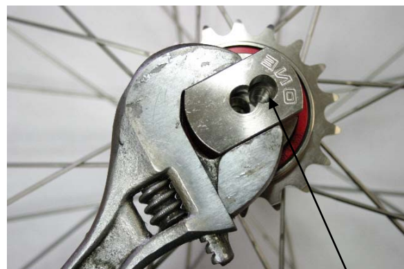
Fig. 2 Thread ENO axle bolt into here.
