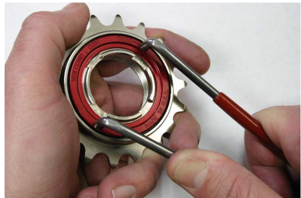
Fig. 21 Tighten lock ring to left.
