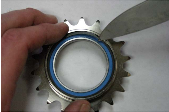
Fig. 8 Removing snap ring.
