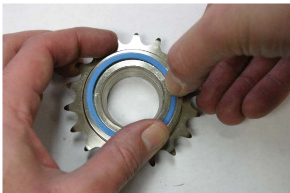
Fig. 22 Push rear seal into place.
