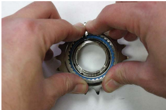
Fig. 14 Seat bearing fully into bore.
