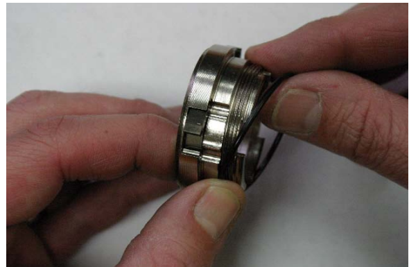
Fig. 15 Install inner driver o-ring.
