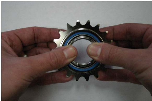
Fig. 5 Pressing out inner driver
