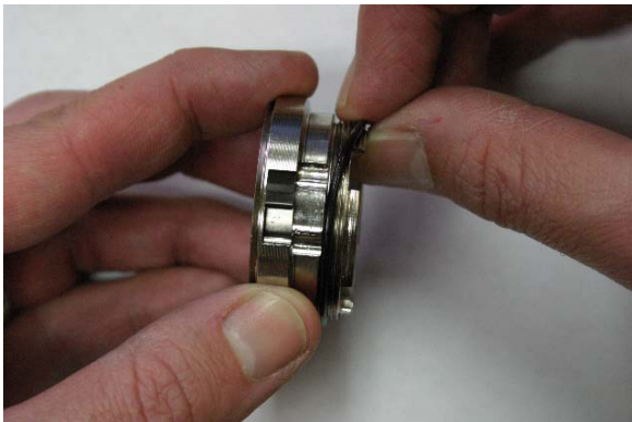
Fig. 10 Remove inner driver o-ring
