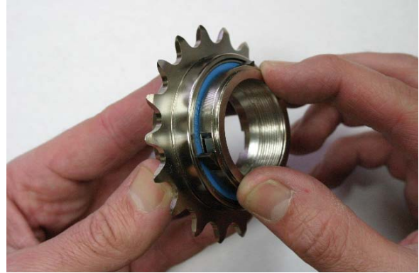
Fig. 13 Place inner driver into bearing.
