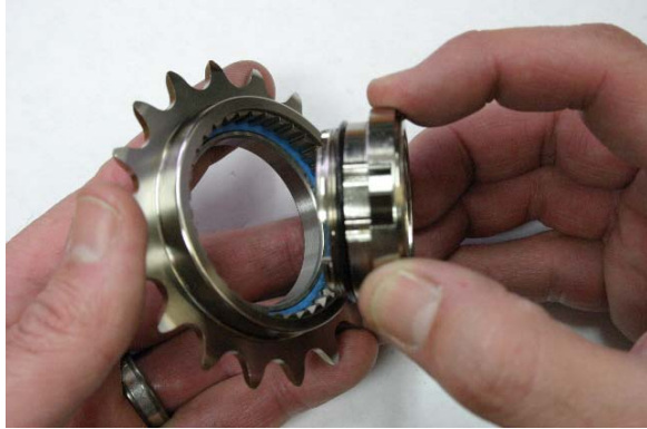
Fig. 18 Insert inner driver into outer gear.
